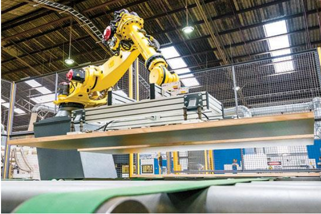
023_Image 8_axis robot lifting and moving the finished doors at Hume Doors.jpg
