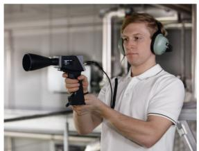
Caption: Identifying and repairing compressed air leaks can generate significant energy savings. 016\_Image 2\_KAESER\_USLD.png
