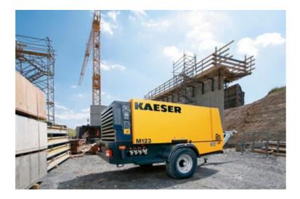
More efficient than ever: The optimised "Mobilair 123" combines a free air delivery of almost 11 m<sup>3</sup>/min at 10 bar with enhanced fuel efficiency.
