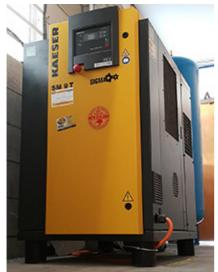
Caption: 3DPrint-AU chose to invest in a Kaeser SM9T series rotary screw compressor with integrated refrigeration dryer, to reliably meet their demand for compressed air.
