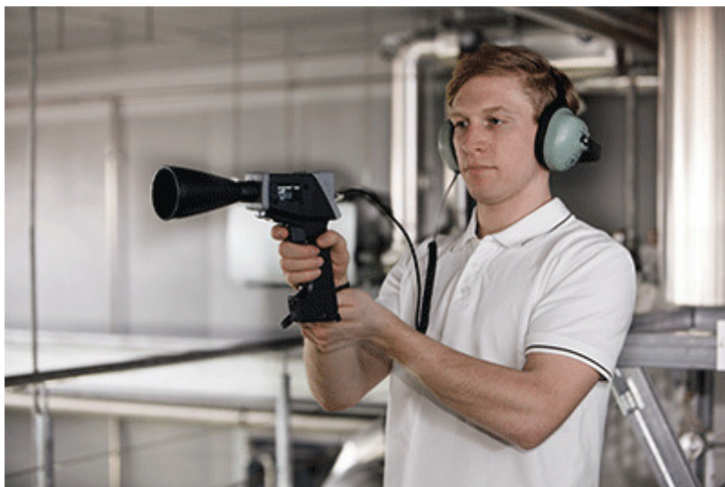
Identifying compressed air leaks with an Ultra Sonic Leak Detector
