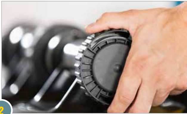
2 The clamping nuts on the cartridge screw connection are then loosened.
