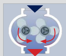
Conveying to discharge side
