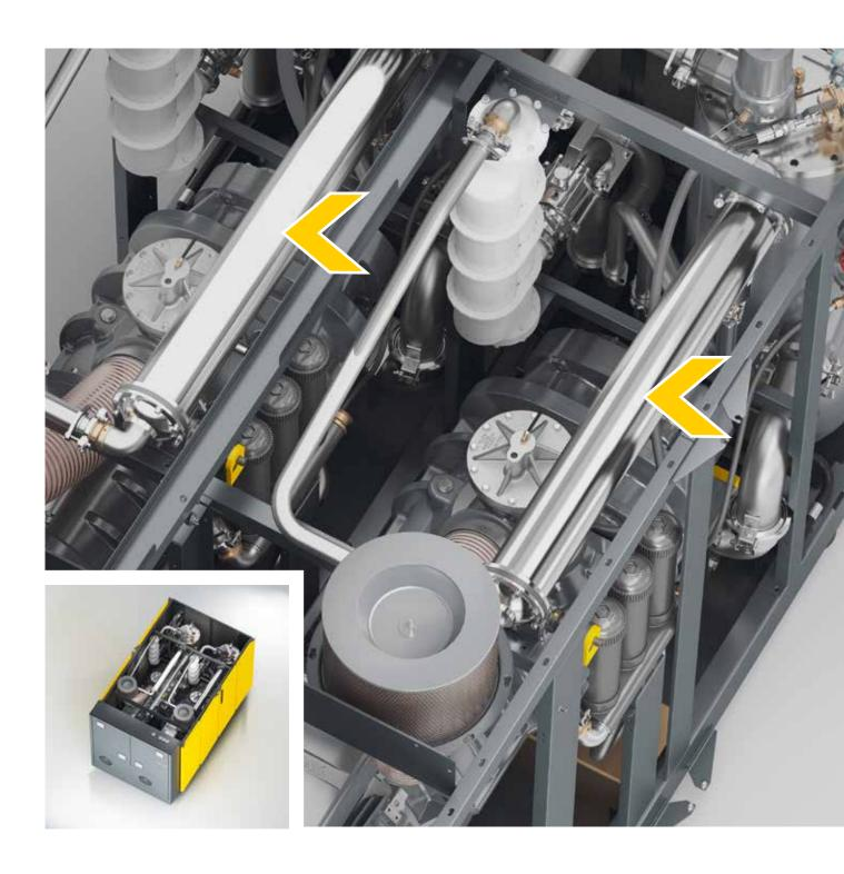
In comparison to plate heat exchangers of adequate cooling capacity, shell and tube heat exchangers made from copper-nickel alloy (CuNi10Fe) are less susceptible to contamination than plate heat exchangers. They are also more robust and the lines and exchangeable inserts can be cleaned very easily. In addition they are seawater-proof, which means that they are suitable for compressors used in shipping operations and operate with minimal pressure loss.
