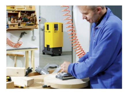
With super-low sound levels of max. 69 dB(A), Kaeser's SXC compact compressed air systems combine outstanding reliability and efficiency with high quality air treatment and a 215-I compressed air receiver.
