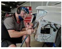
Caption: Compressed air is an essential utility at Charlie Battisti. It is used extensively, from powering the air tools - such as the sanders and polishers - to providing air to the dedicated paint refinish facility.
