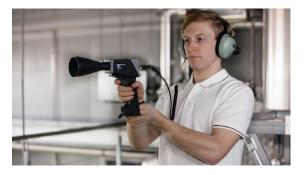
Caption: Detecting and fixing compressed air leaks has an overall energy savings potential of 6-10 percent.
