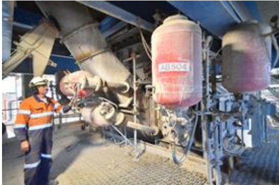
Caption: Compressed air is an essential utility required throughout the cement manufacturing process, from facilitating the flow of materials from start to finish, to assisting with the actual manufacturing process itself. Pictured above some air cannons.
