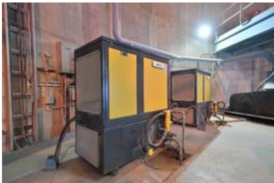
Caption: The existing Kaeser compressors that were already onsite and working reliably at Golden Bay Cement.
