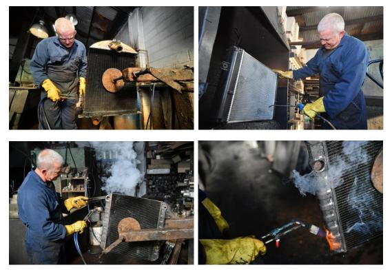
Caption: From cleaning radiators with a bead blaster, to using gas torches for welding - compressed air is an essential utility used and relied upon every day in Trevor French Radiators' workshop.
