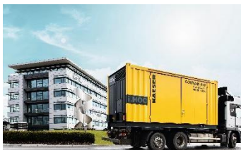
Caption: A complete compressed air system, including treatment in a mobile container solution.
