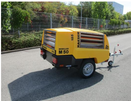
Caption: Prototype of the diesel powered Kaeser M 50 including aquaculture modifications
