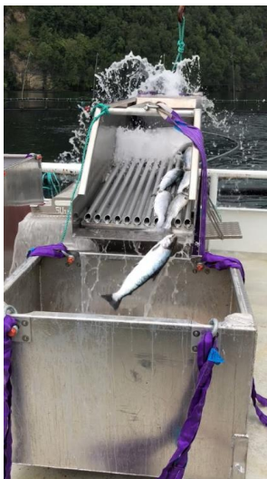
Caption: Separation of carcasses and water in the morts removal process.
