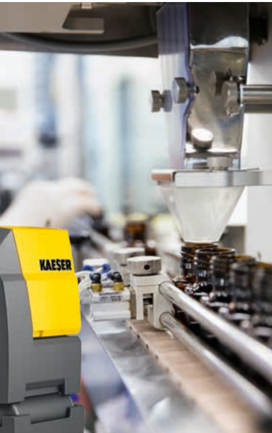
Compressed air is used for the packaging process.
